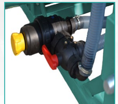
Filter za samopunjenje Intake filter predisposed for self-filling
