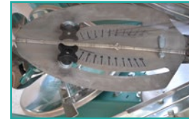
Skala za podešavanje preciznog rasipanja Setting gauge corresponding to the spreading charts for highly accurate fertilization
